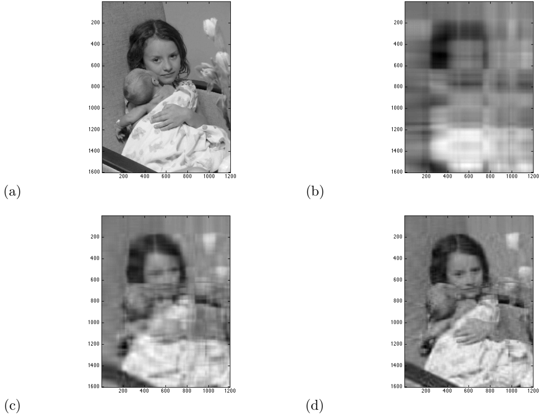
FIGURE 1. Low rank approximations of image. (a): original; (b): rank 3; (c) rank 10; (d) rank 20.
